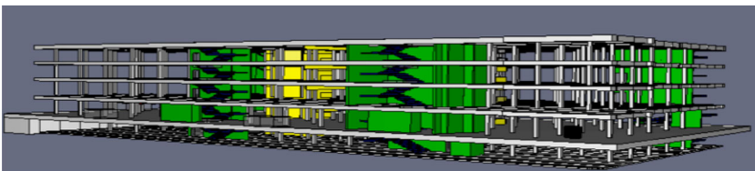
Figure 5. 3D model of the five storey shopping mall (green are staircases, yellow are central voids) (Color figure online).
