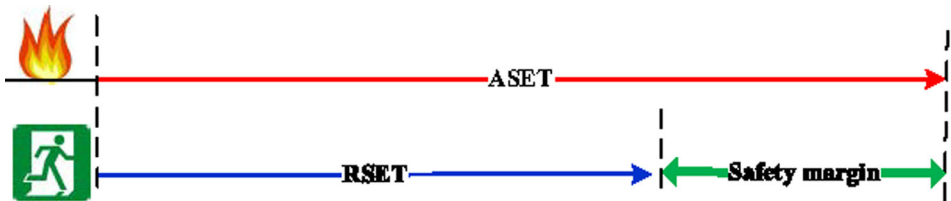
Figure 2. The traditional deterministic timeline of estimating the casualties in building fires.
