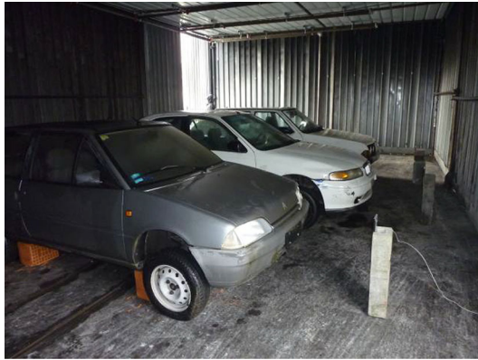
Figure 3. Car arrangement within the test chamber; nozzles and piping are also visible in this photo, below the ceiling; plate thermometers are also visible in front of each car.
