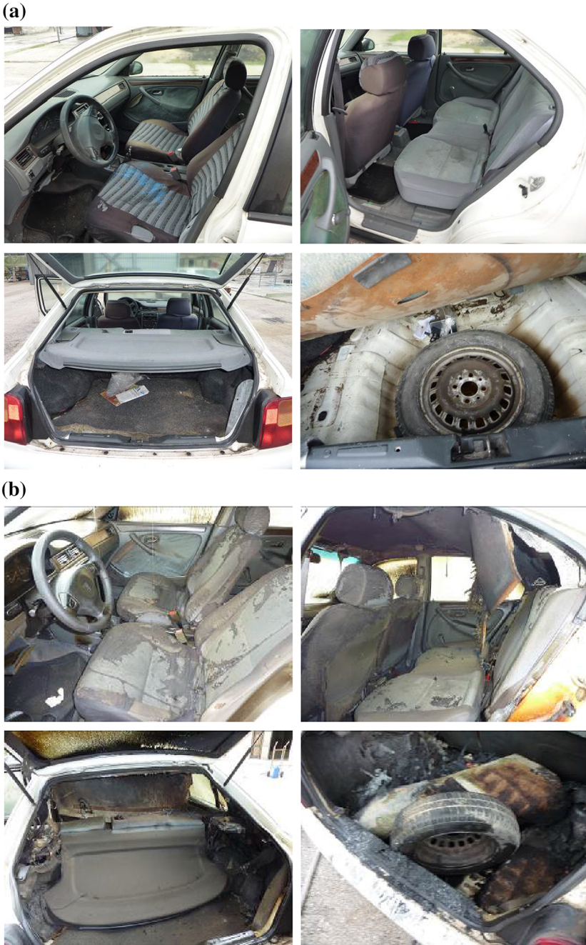
Figure 6. Photos of the interior of the central car used in test C1SPK: (a) before and (b) after testing.
