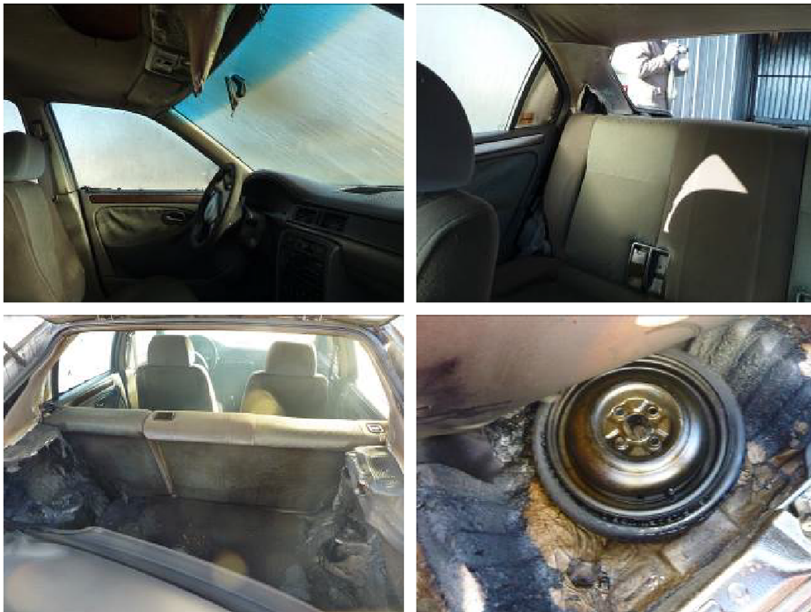
Figure 7. Photos of the interior of the central car used in test C1WM1.5: (a) before and (b) after testing.
