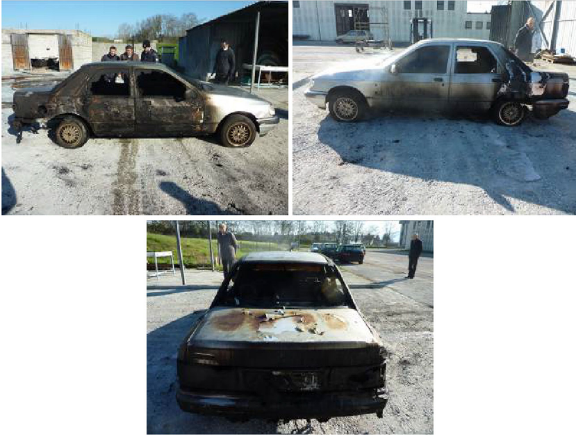
Figure 11. Photos of the exterior of the central car used in test C2WMA after testing.
