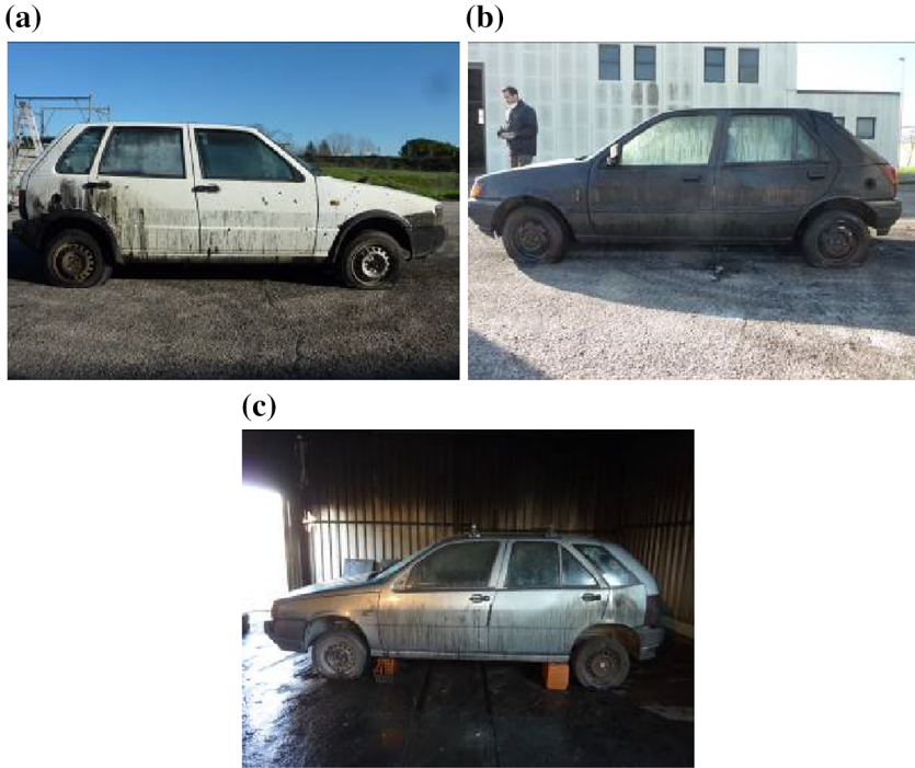
Figure 8. Photos of the exterior of (a) Target 1 car used in test C1WM1.5, (b) Target 2 car used in test C1WM1.5 and (c) Target 2 car used in test C1WM2.0 after testing.
