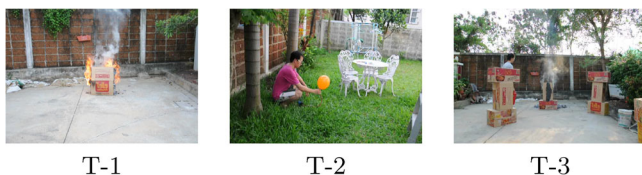
Figure 4. Sample frames from training videos used for adjusting thresholds for QuickBlaze. T1 has 7343 frames, T2 has 1607 frames, and T3 has 3383 frames. T1 and T3 contain both fire and smoke regions, while T2 contains no fire or smoke but does contain an orange balloon as a distracter (Color figure online).
