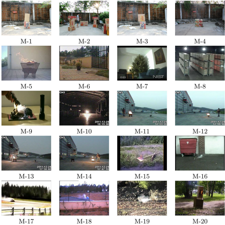
Figure 5. Sample frames from test videos that contain flame or smoke. In each case, the first frame containing flame or smoke according to human observations is shown. Although M-1, M-3, and M-4 are similar to videos in the training set, they were acquired at different times with different target objects.
