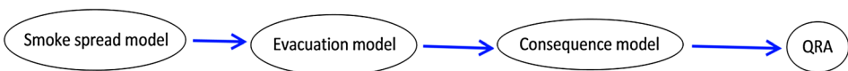
Figure 6. Illustration of how the sub-models lead to a QRA. Input for the scenarios is obtained from the bow-tie branches as explained in Figures 2, 3 and 4.
