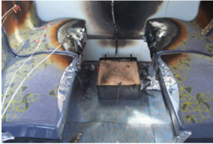
(b) view of seat and wall. The falling object is a polycarbonate light diffuser softened during test
