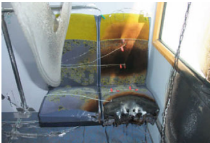
Figure 22. View of burnt areas after the real-scale test according to scenario 1A. (a) view of the burner and seats after test, (b) view of seat and wall. The falling object is a polycarbonate light diffuser softened during test, and (c) view of the window and wall panel.
