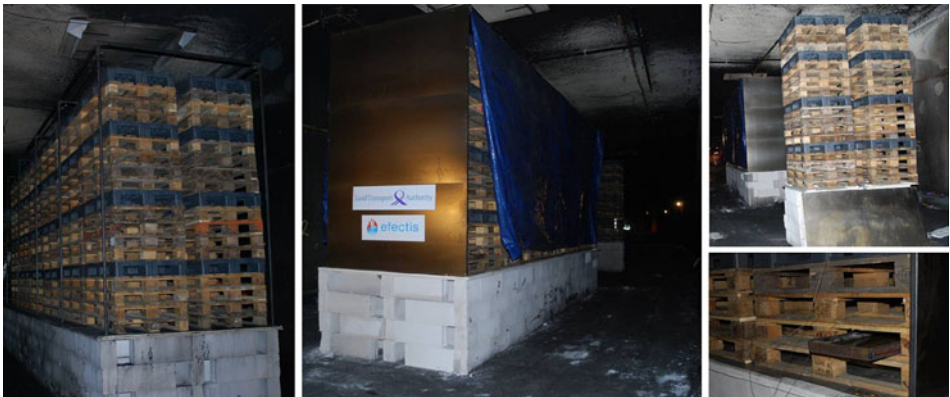
Figure 4. Photographs of fire load (left-before covering, center-as used in the fire test, upper right-target array and lower right-ignition tray).
