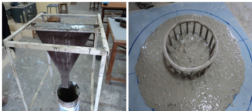
Figure 1. Workability Test on Fresh SCC.
