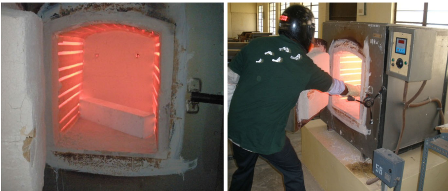
Figure 2. Heating of SCC Specimens at 900°C.
