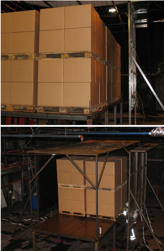
Figure 1. The trailer mock-up without (top photo) and with a roof. Note that a smaller amount of commodity, two instead of six rows, was used for the tests with the roof. Steel screens instrumented with thermocouples were placed on both long side of the mock-up.
