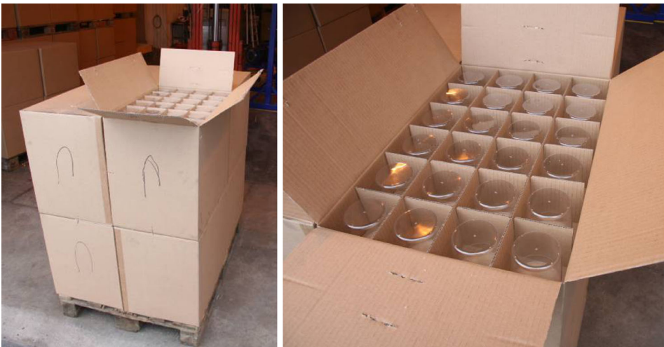
Figure 2. One pallet load of the EUR Std plastic commodity (left) with a close-up photo of the arrangement of the plastic cups in the individual cartons (right).
