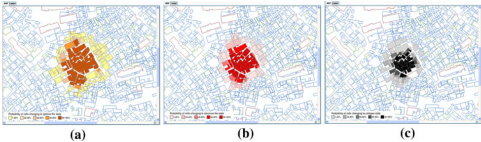
Figure 11. Three types of probability maps after 3-h fire-spread simulation. (a) Ignition probability map, (b) structure-fire probability map, and (c) collapse probability map.
