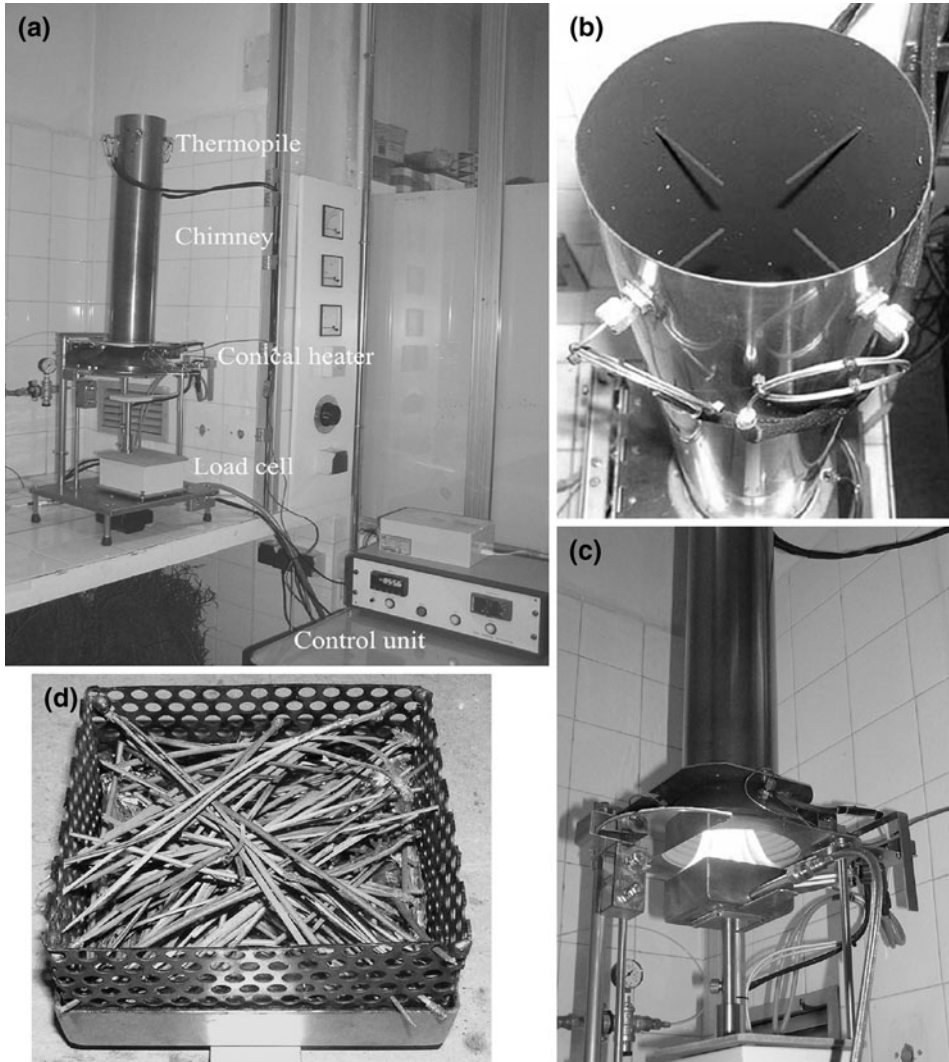
Figure 1. a General view of the MLC device. b Detail of the thermopile. c Detail of methane burner used to calibrate thermopiles. d Porous holder with Pinus pinaster dead litter, immediately before a test.
