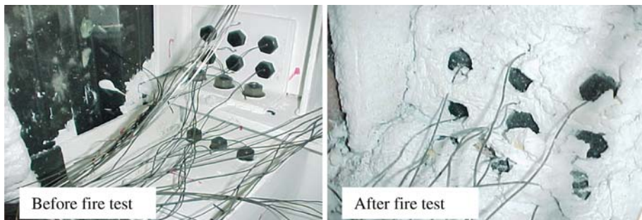
Figure 8. Unprotected bolts in protected web cleat before and after 60 min fire exposure (test SP2).
