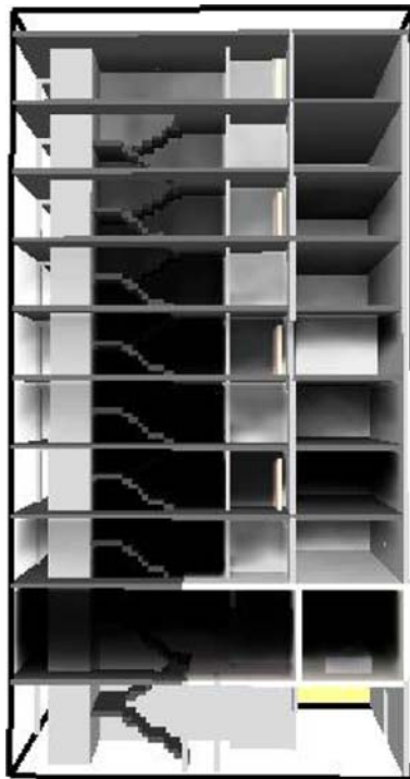
Figure 13. Smoke movement of test PP2.
