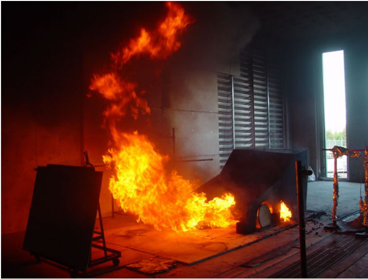
Figure 2. Pool fire underneath a vehicle.
