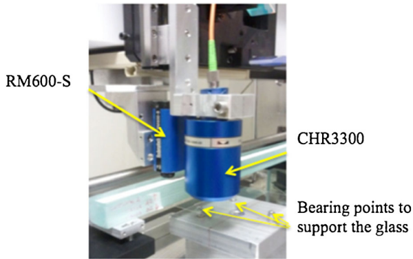
Fig. 4 Setup for 1D profiles measurements: the CHRcodile 3300 sensor head mounted on the LTP and the RM600-S sensor measuring the calibrated rod to subtract the LTP stage errors. The glass is supported horizontally on three points
