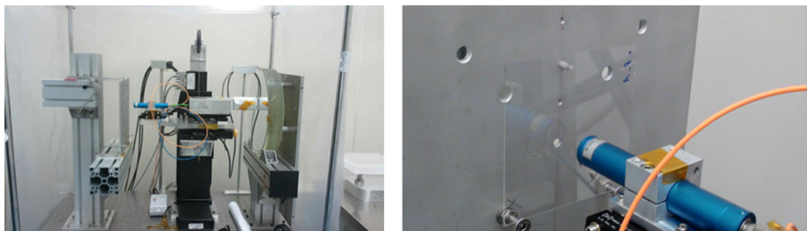
Fig. 5 Setup for the 2D profiles measurements. Left : the CUP setup. Right : the CHRcodile 660 sensor head mounted on the CUP. The glass is supported vertically on three points
