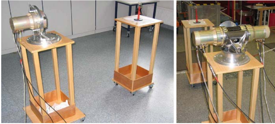
Fig. 5 Detector holders with NaI ( left panel ) and BGO detectors ( right panel ) are positioned in front of the radioactive source (on top of the red holder) on their wooden stands during the calibration at the MPE laboratory
