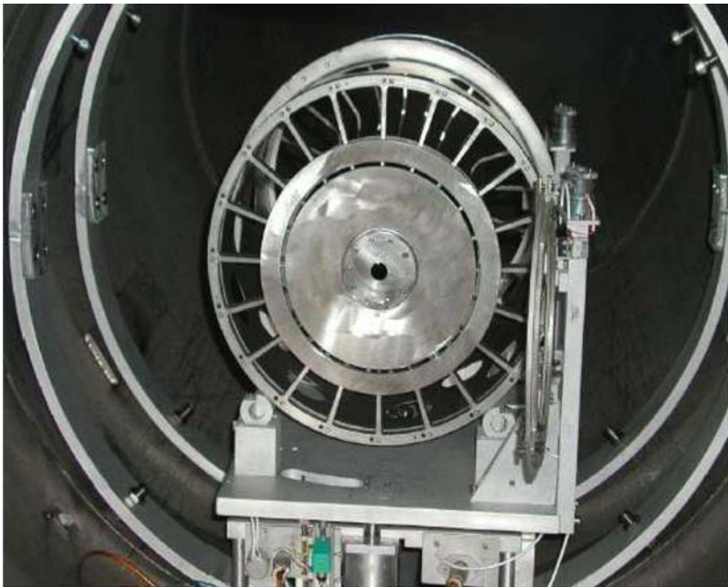
Fig. 4 Spider module holding one multilayer coated mirror shell (at the ring), the shutter door is seen at the right of the module, the hole in the centre is used for flat-field measurements (a shutter at the back of the module allows to open/close this central hole) [9]
