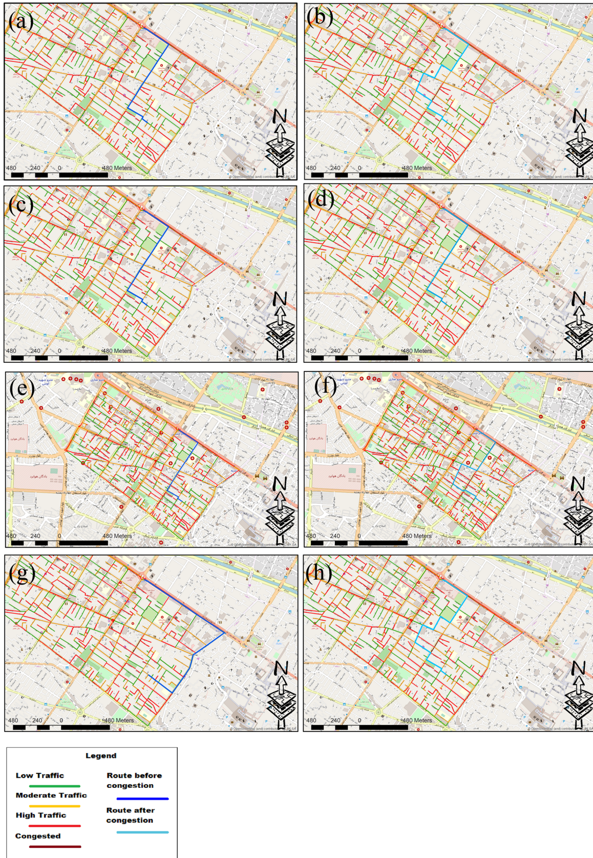
Fig. 6 Optimal routes obtained from the algorithm a, b AS-gamma c, d AS-MON e, f AS-IMG g, h AS-Restart
