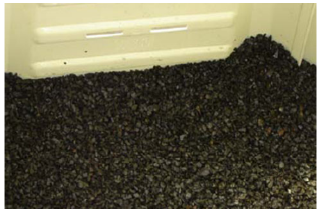
Fig. 3 Different sizes of gravels used in preparation of the vermifilter bed (upper layers gravel sizes 10–12 mm)
