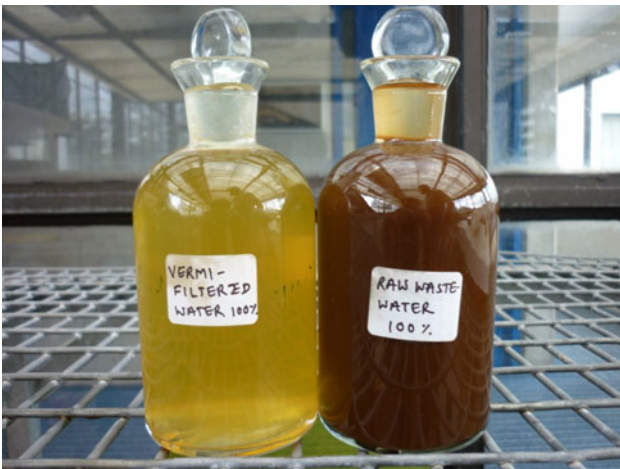
Fig. 5 The dark-brown raw petroleum wastewater (right) color changes into a pale yellow (left) after vermifiltration (Color figure online)
