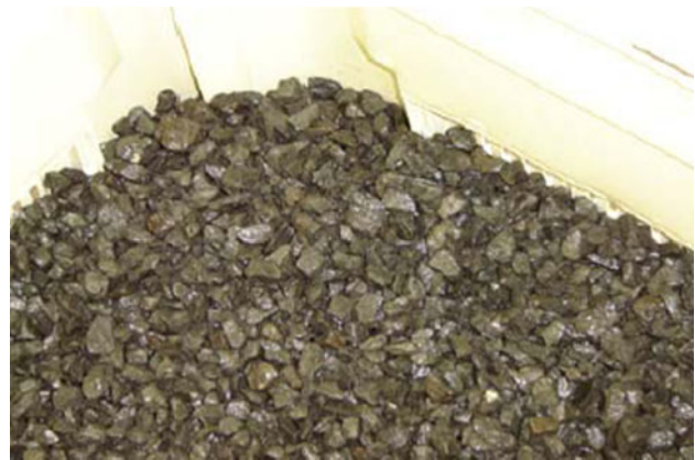
Fig. 2 Different sizes of gravels used in preparation of the vermifilter bed (middle layer gravel sizes 3.5–4.5 cm)
