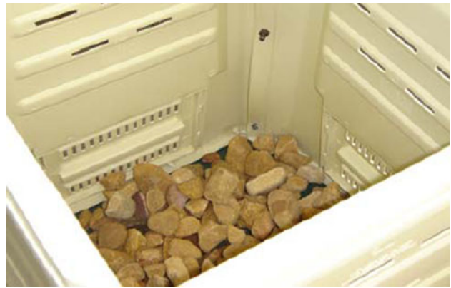
Fig. 1 Different sizes of gravels used in preparation of the vermifilter bed (bottom layer gravel sizes 7.5 cm)
