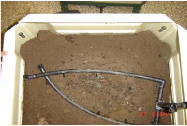
Fig. 4 Soil bed with earthworms in the uppermost layer & the device of wastewater discharge and distribution through perforated PVC pipes
