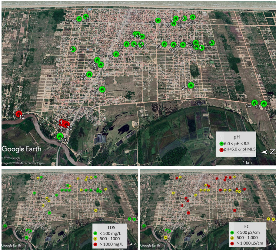
Fig. 3 Map of infractions for pH and TDS against MPV and distribution of EC values
