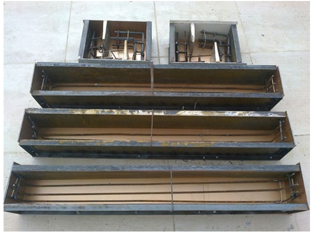
Fig. 6 View of molds used for beams and push-off specimens (current investigation)
