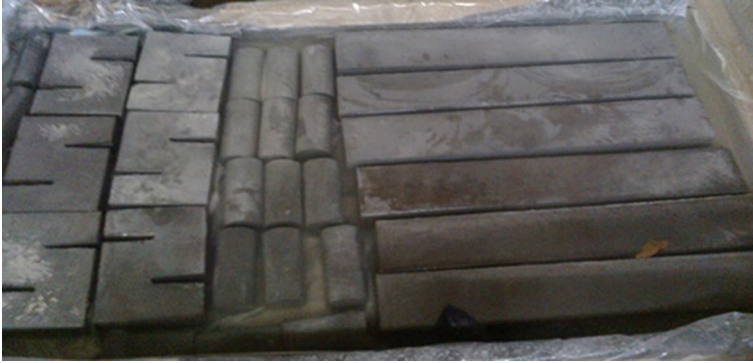
Fig. 8 Specimens inside water tank for curing (current investigation)
