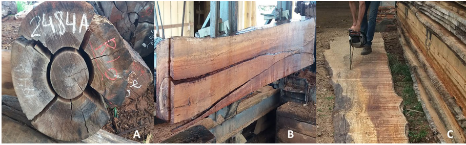
Fig. 3 a, b Logs with presence of cracks; c sapwood removal with chainsaw for discard
