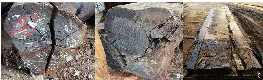
Fig. 4 a, b Eschweilera coriacea log with cracks; c Sawn boards of E. coriacea
