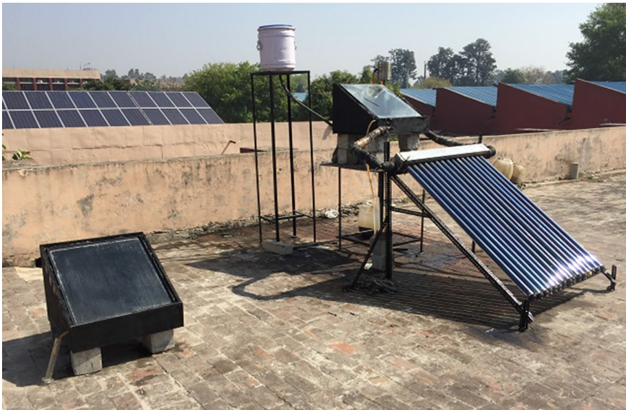
Fig. 17 Photograph of simple basin type solar still and evacuated tube-integrated solar still
