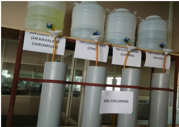
Fig. 3 Wastewater feeding arrangement
