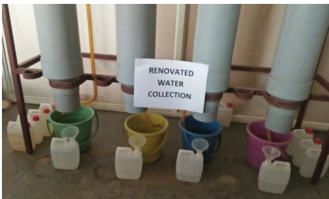
Fig. 4 Wastewater effluent collection system
