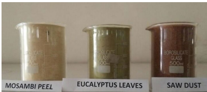
Fig. 5 Adsorbents of SAT simulation
