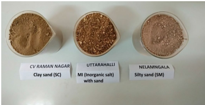
Fig. 2 Soil samples of SAT
