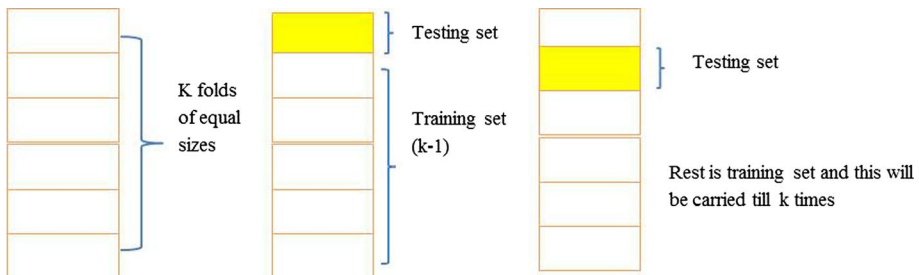
Fig. 3 k -fold cross-validation and every time random fold is selected as testing set
