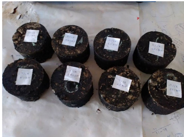
Fig. 7 Marshall specimen sampling for testing
