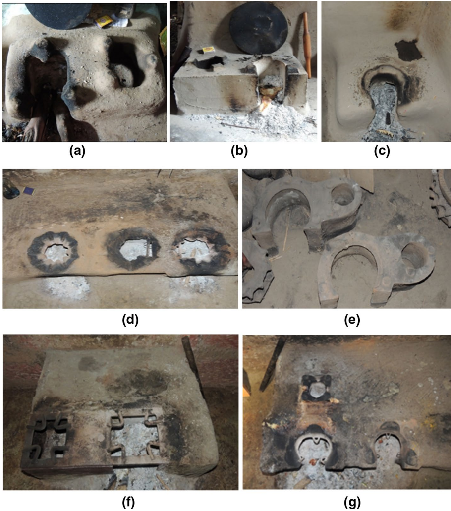
Fig. 2 Different types of cookstoves from the field. a Traditional stove, b Cement stove, c Sobna stove, d Lotus shape stove, e Khapar stove, f Iron reinforced stove, g Traditional (in-line) stove
