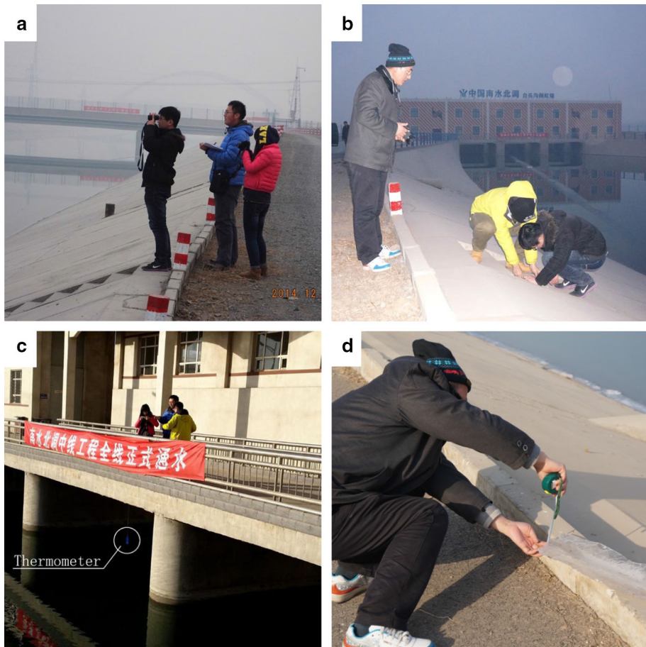
Fig. 2 Channel profiles, water temperature and ice thickness were measured on site: a measurement of the channel length and width with laser range finder, b measurement of the channel slope with an angulometer, c observation of the water temperature using a thermometer tied to a stone and d investigation of the thickness of the ice collected from the thick ice layer
