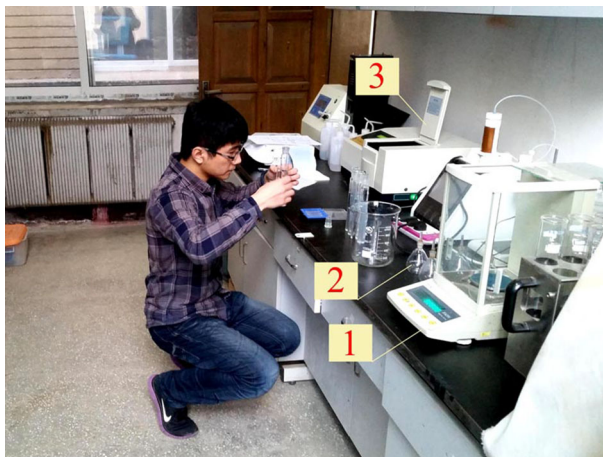
Fig. 3 Instruments used in the experiments on water quality analysis. 1 FA214 electronic balance, 2 pycnometer and 3 UV-7504 spectrophotometer
