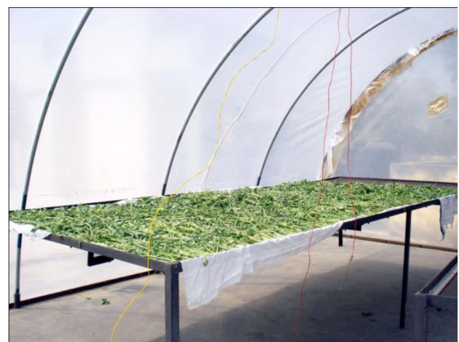
Fig. 2 Inside view of solar dryer with drying product
