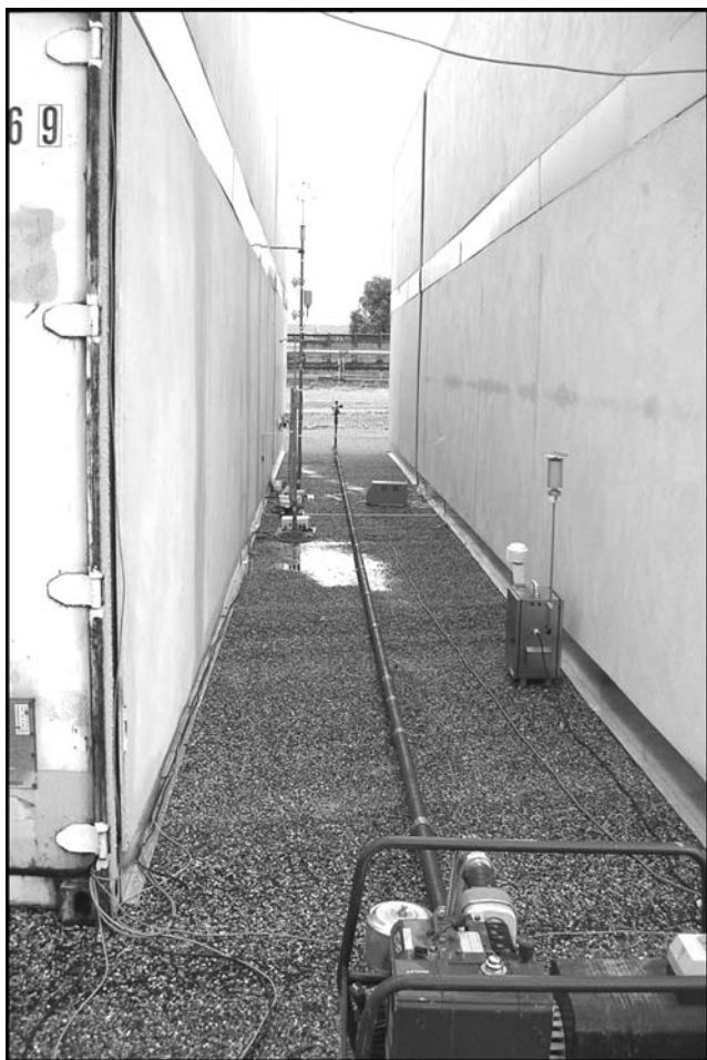
Fig. 2 Perforated tube used as a line source of emissions inside the 2nd consecutive street canyon
