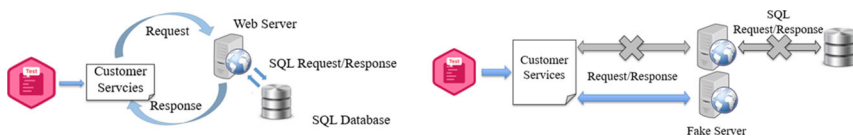
(a) Test Dependencies on Web Server and (b) Dependency Isolation by an Mock Object SQL Database
