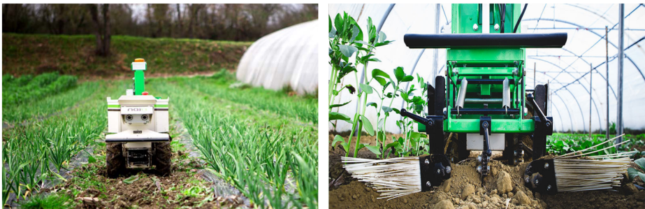
Fig. 1 Oz in operation. Left: front view; right: back view with tools
