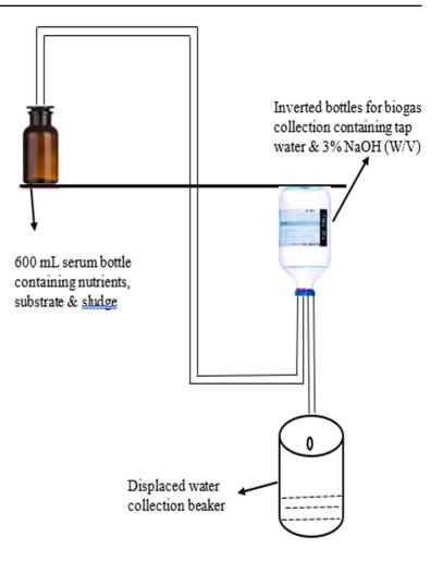
production was monitored after every 24 h using the water replacement method and the volume of biogas produced in each reactor was recorded. In order to assess the effectiveness of the anaerobic digestion process, the routine parameters including pH and temperature were also monitored regularly. All the experiments in the present study were carried out in triplicate samples and average of the close two values were reported in the results.
