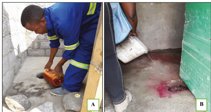
Fig. 5 A Dosing of fluorescein and B dosing of rhodamine in pit latrines upstream of observation springs
