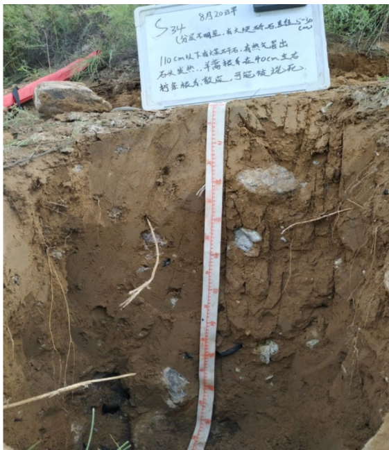
Fig. 7 Profile method to verify the gravel content of the sample (profile P 4 )
