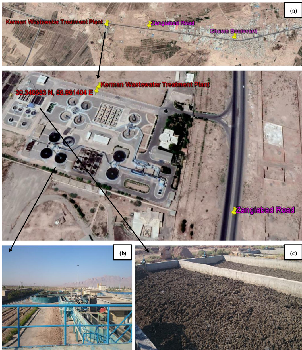
Fig. 1 (a) Study area location; (b) general scheme of Kerman WWTP; and (c) sludge drying beds
