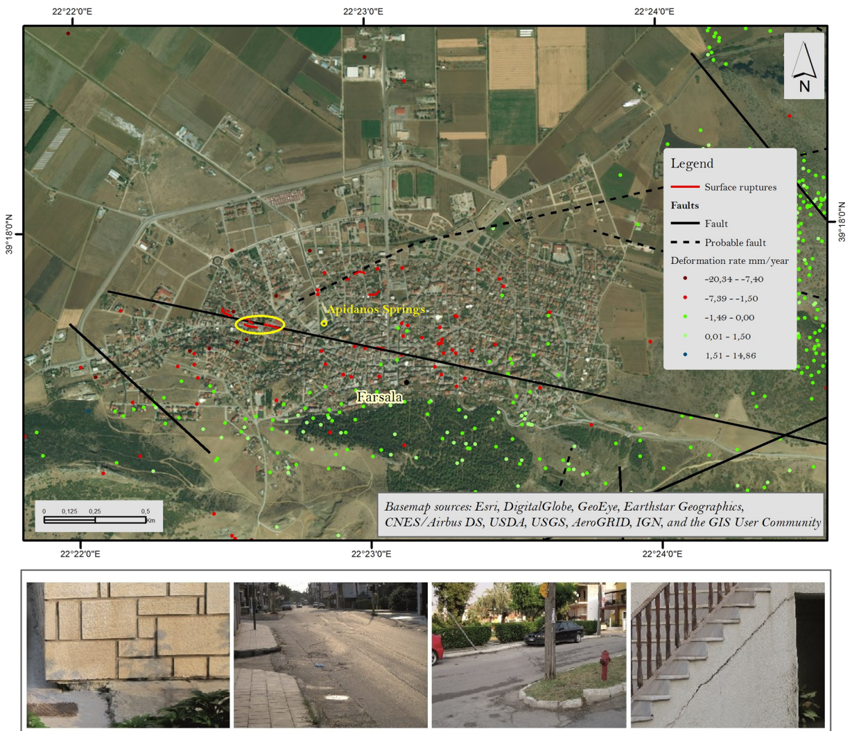
Fig. 9 The spatial distribution of the surface ruptures and PSI data. The pictures at the bottom of the figure illustrate damages on the road network and buildings located inside the yellow eclipse
