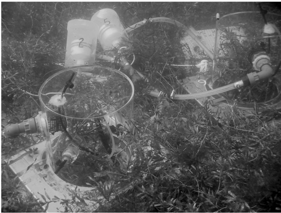
Fig. 1 Close-up of the in situ chambers deployed over an Amphibolis antarctica bed to quantify uptake rates of phosphorus. Three chambers each were deployed simultaneously over Posidonia angustifolia and Amphibolis antarctica beds. The chambers were bolted on to stainless steel cutters deployed on the seagrass bed 24 h prior to the experiment. The water in the chamber was circulated with a submersible inline pump through a pressure compensator. Sampling ports on the chamber facilitated spiking of nutrients and collection of water samples
