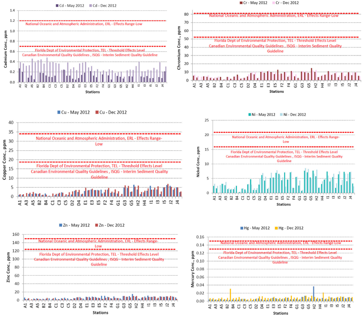
Fig. 6 Cd, Cr, Cu, Ni, Zn and Hg concentrations from sediment samples of Doha Bay during May and December 2012 compared with international standard recorded
