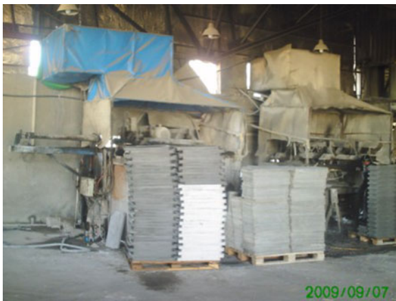
Fig. 1 Cutting process for AC sheet manufacture
