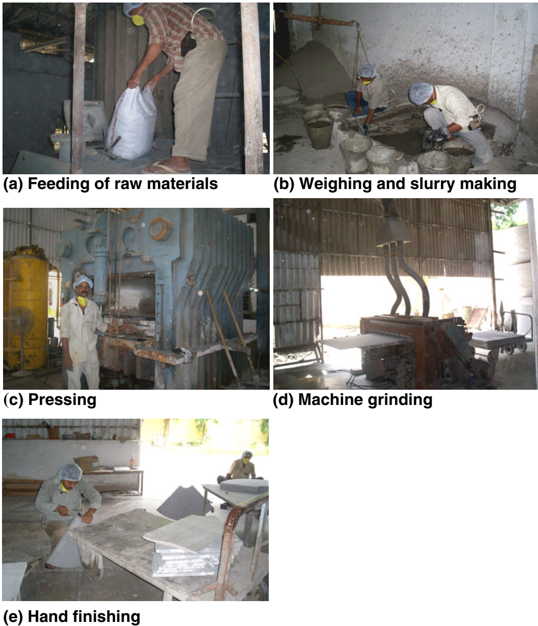
Fig. 1 Manufacturing process for thermal insulating boards. a Feeding of raw materials, b Weighing and slurry making, c Pressing, d Machine grinding, e Hand finishing
