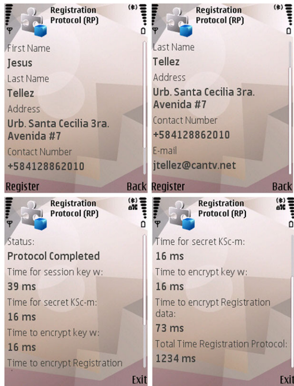
Fig. 11 Snapshots of CCMS-VAN wallet during the execution of the Merchant Registration Protocol phase on Nokia™ N95 device
