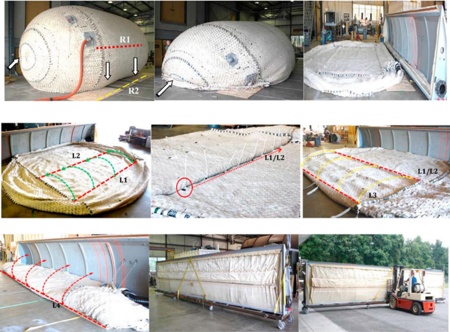
Fig. 8 Inflatable Plug: Folding and packing sequence [117]
