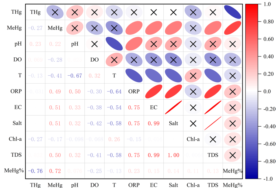
Fig. 4 Correlations between environmental factors and different mercury chemical species in water of Wuliangshuai Lake
