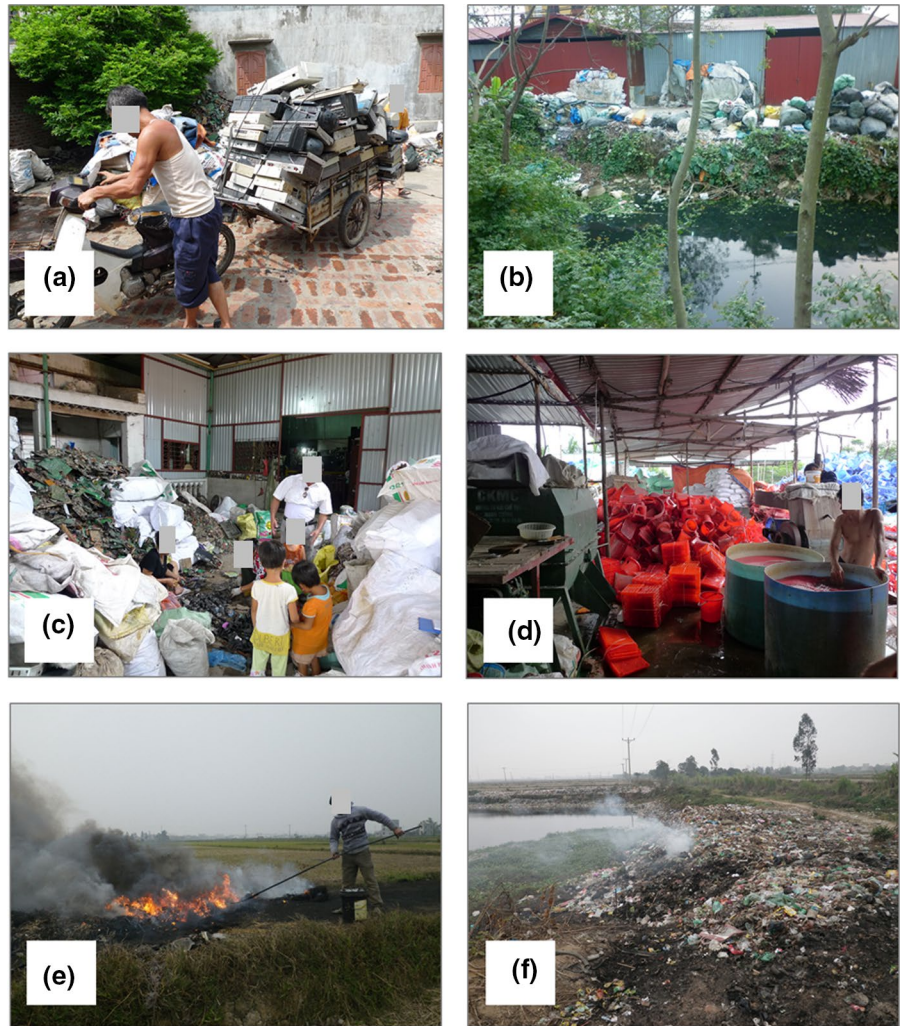
Fig. 2 Typical e-waste processing activities in Bui Dau, northern Vietnam: a collection; b stockpiling; c manual dismantling; d plastic recycling; e open burning of wires and cables to recover metals; f open burning of less valuable materials and domestic waste
