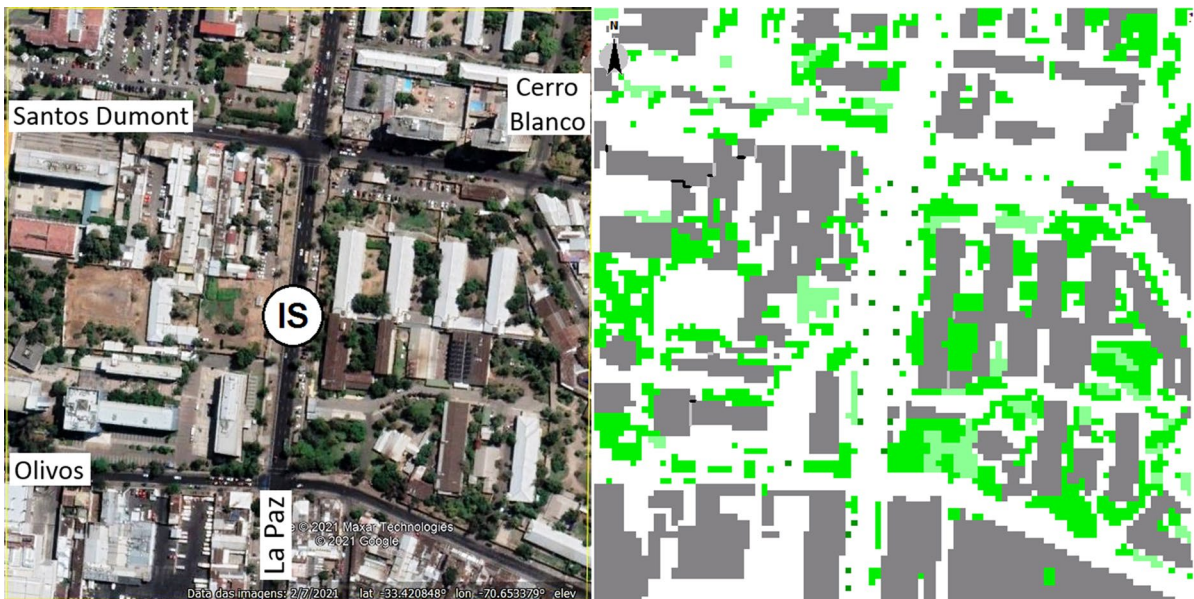
Fig. 4 Aerial view and modelled land use and cover at the Independencia municipality (location of the ORMS-IS). Building blocks (grey) cover 33% of the surface, bare land (white) 47.6%, trees (dark green) 15.8%, and grass (light green) 3.3%, respectively
