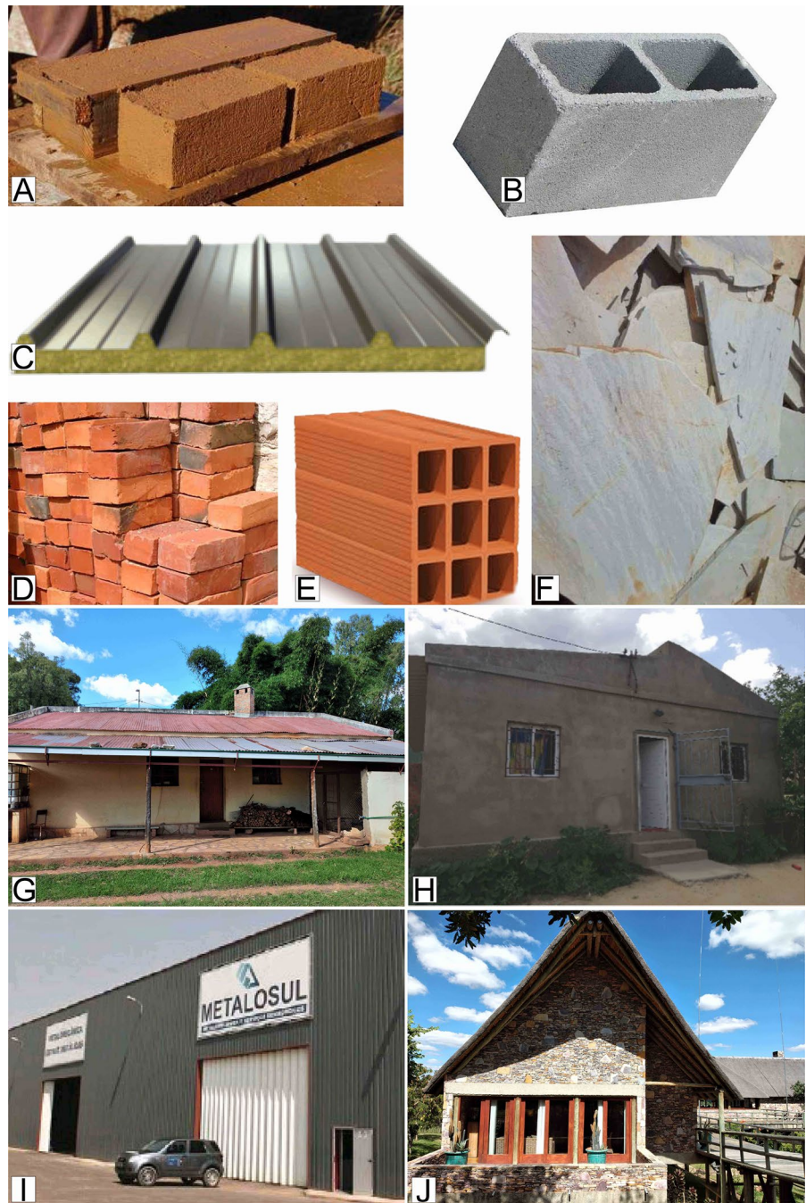
Fig. 2 Examples of building materials and styles: A Clay (Adobe); B Concrete block; C Metal (Metallic plates); D filled clay brick; E hollow clay brick; F Stone; G Adobe built housing; H Dwelling built with concrete blocks; I Construction with metal plates; and J Dwelling built with stones
