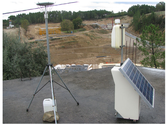
Fig. 9 Cunha Baixa uranium mine a dosimeters and dust meter placed in the terrace of a house located nearby the mine during rehabilitation works
