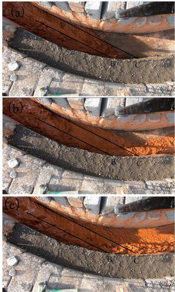
Fig. 7 debris flow erode concave bank at different time
