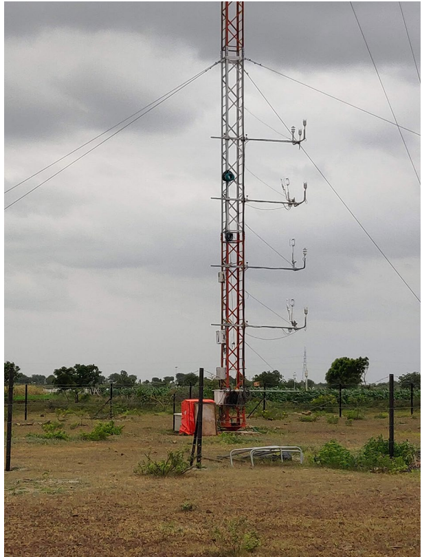
Fig. 1 A partial view of the 50-m instrumented tower, looking towards the South. The booms where the instruments are mounted face towards the West. The fetch area at the South-West sector of the tower includes scattered trees and bushes, representing a typical site
